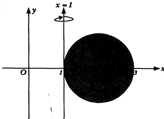
In the diagram above, the circle  $(x - 2)^2 + y^2 = 1$  is drawn. The region bounded by the circle is rotated about the line  $x = 1$ .
